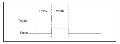
The following figure shows how to create a high and low pulse train with a microsecond delay and width.
